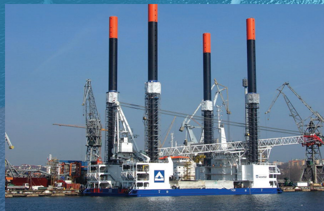
Fig 3: JACK-UP BARGE B392 "THOR" (Source: www.crist.com.pl )
